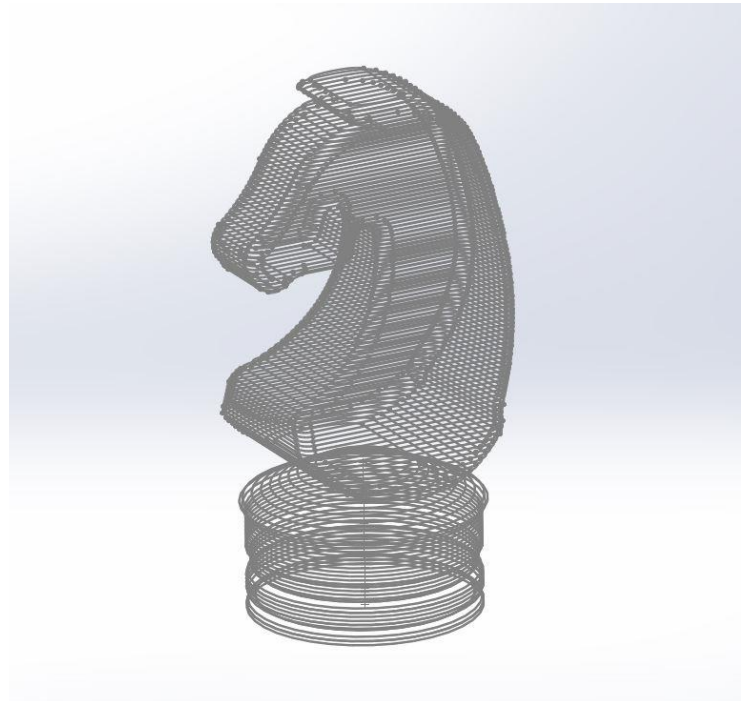
Slicing the input part to calculate cross sections
